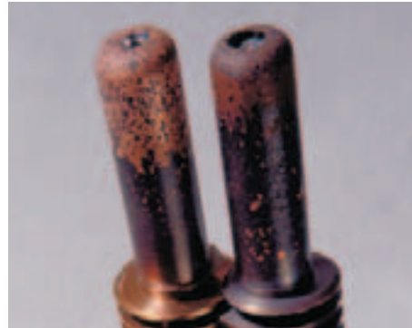
Electrode after normal use, electrode after excessive use
